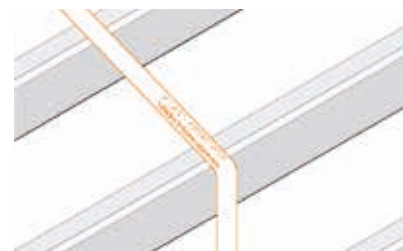
Tactile information on a handrail
